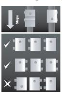
If the ColorGard assembly utilizes the VersaClip for attachment of the ColorGard crossmember, the bolt hole in the clamp should be at the upslope end of the clamp. If the assembly uses punched ColorGard without VersaClip the hole should be at the downslope end of the clamp. When using the S-5-U, determine which side of the clamp to load the setscrews into, and thread the setscrews into all clamps, being careful that the bolt hole will be in the correct (upslope
